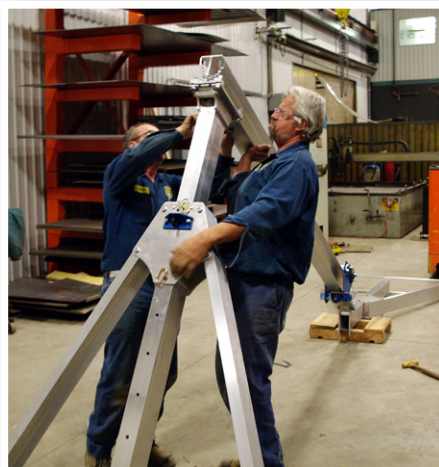
Aluminum gantry crane when folded for storage.
